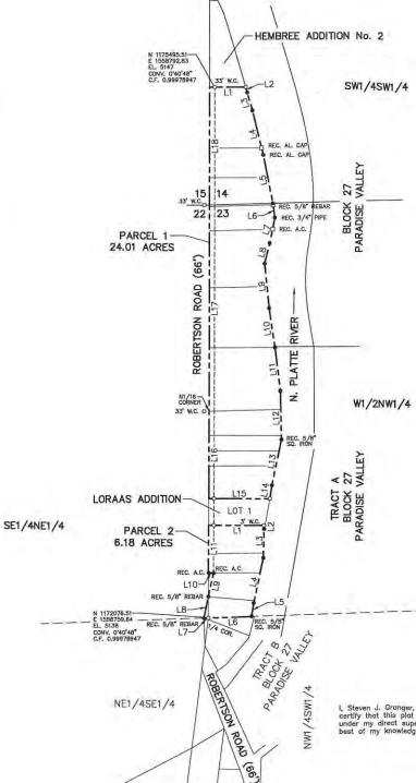
Parcel 1 - Line Table Line # Direction Length L1 S89'58'57"E 232.67" L2 S16'01'14"E 37.00' L3 S16\*20\*22\*E 120.58\* L4 S13'48'37"E 294.60" L5 S11"10"23"E 317.30" L6 S7'57'23"E 94,64" L7 S11'42'58'W 167,42' LB S14'08'58"W 135.44" L9 S5'40'02"E 287.52" L10 S8'39'02"E 257.09' L11 S6'53'02"E 282.01" L12 S117'02"E 314.39" L13 S11'57'03"W 300.37' L14 S9'02'27"W 87.87" L15 N89'42'01"W 395.50' L16 N015'44"E 562.35' L17 N010'26"E 1328.68' L18 NOTO'37"E 759.63"
